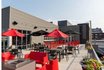
Installed using a pedestal system, the pavers form even joints that direct storm water away from their surface, allowing for proper drainage. Skylands Concrete Deck Pavers protect the roof membrane from UV rays and simplify maintenance, as each unit can be removed.
