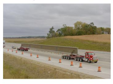
During production, each prestressed girder is manufactured to specification and arrives ready to be installed upon delivery.
