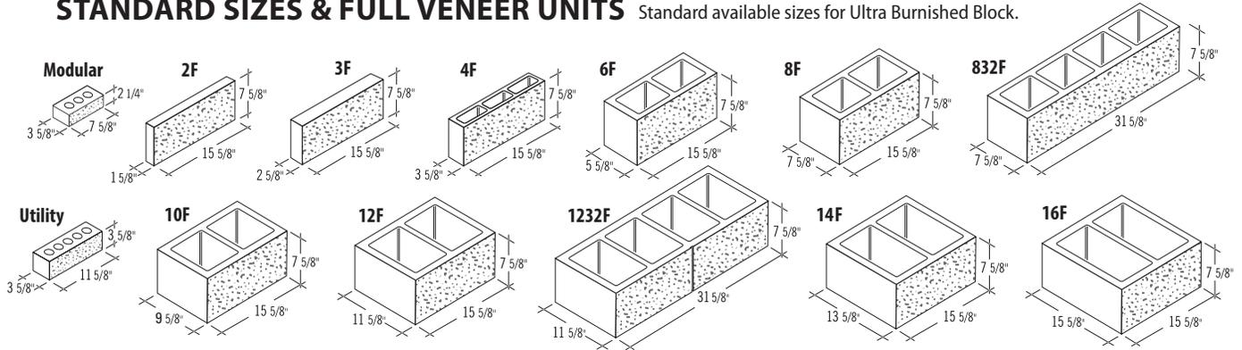
The following shapes, finishes, corner arrangements, etc. are available for the standard sizes (2", 3", 4", 6", 8", 10", 12", 14" and 16") for the Ultra Burnished Block shown above.
