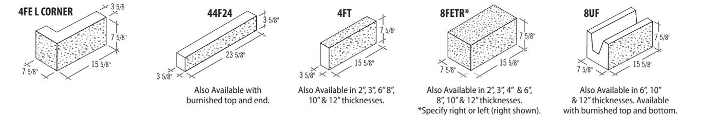
The following shapes are available with burnished tops and ends. A bullnose can be added (at top or end).
