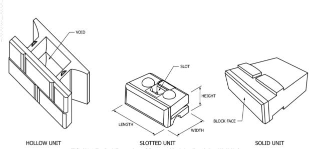
FIG. X1.1 Typical Examples of Precast Modular Retaining Wall Units
