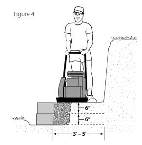
Retaining walls require only a certain amount of compaction with hand-operated equipment to consolidate the soil and minimize settling. Excessive compaction can cause forward rotation of the wall facing. Large equipment operating too close to the wall may cause over-compaction and result in localized bulging. It can also damage geogrid reinforcement materials.
