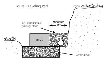
drainage rock until it is level with the top of the first course. Compact the fill with a hand-operated plate compactor on both sides of the first course to required specifications, or to 95% of maximum Standard Proctor Density (a method used to determine compaction). Compact on top of the block, and clean the top of the first course units to begin installation of second course.
